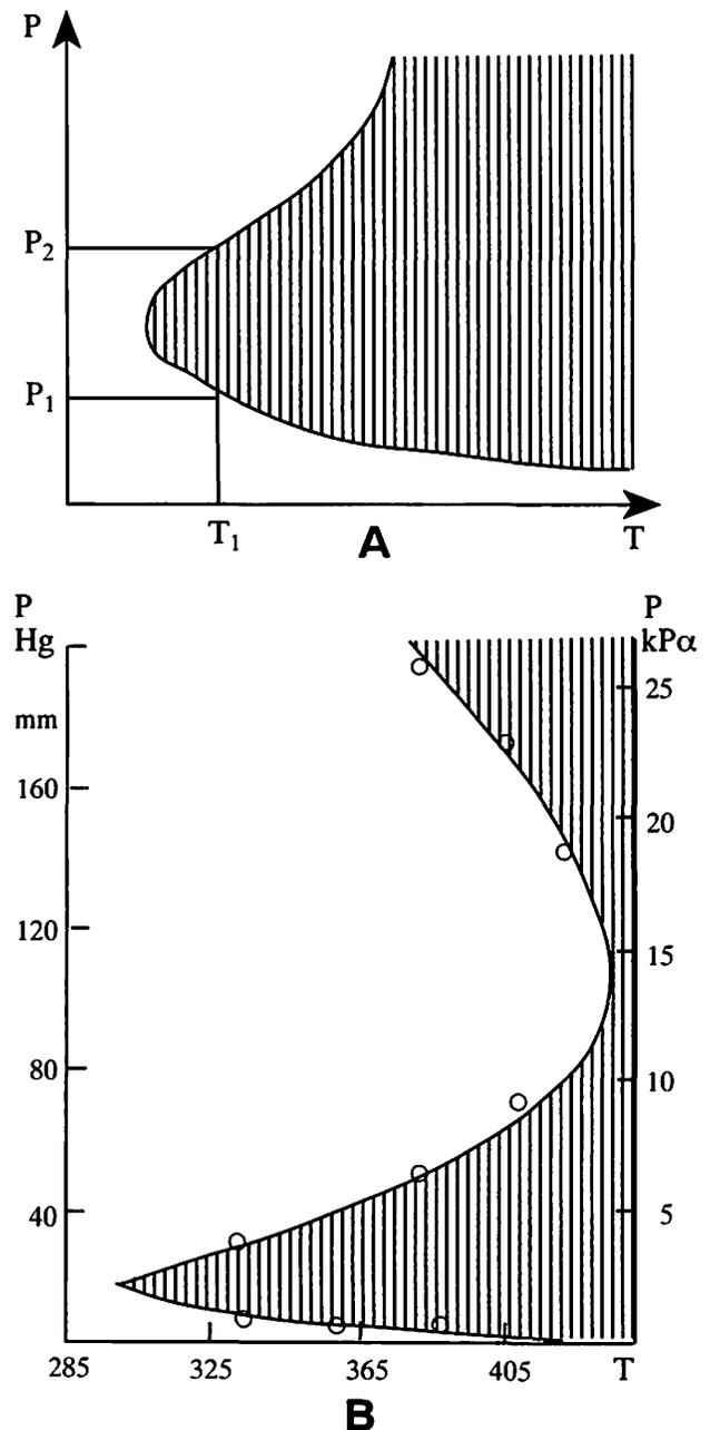
Figure 6. Limits of spontaneous combustion under different pressure/temperature conditions: A – theoretical; B – for hydrogen sulfide ( $\text{H}_2\text{S}$ ) (from Panchenkov and Lebedev, 1974).
